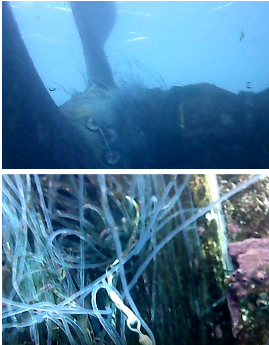
Figure 7: Propeller and Shaft of M/V “DEIMOS” wrapped in fishing gear. Source: Videos - Dive Operation
